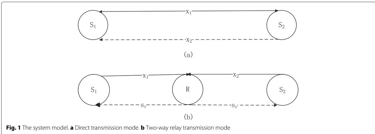
**Fig. 1** The system model. **a** Direct transmission mode. **b** Two-way relay transmission mode
