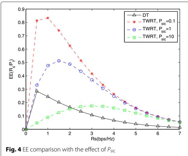
Fig. 4 EE comparison with the effect of  $P_{\text{sic}}$
