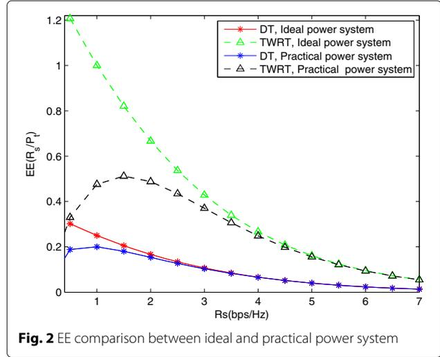
**Fig. 2** EE comparison between ideal and practical power system
