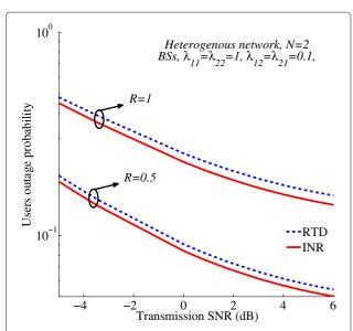
**Figure 6 Outage probability vs the transmission SNR 10 \log\_{10} P.** Heterogenous network N=2, a maximum of M=1 retransmission rounds. The fading parameters are set to  $\lambda_{1,1}=\lambda_{2,2}=1$ ,  $\lambda_{1,2}=\lambda_{2,1}=0.1$ . The same outage probability as in the RTD scheme is achieved by repetition codes with repetition order of 2.
