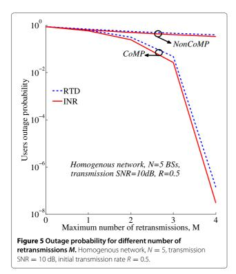
transmission rates. As shown in the figure, CoMP transmission leads to considerable outage probability reduction, particularly at low rates. Moreover, the difference between the performance of the RTD and INR protocols increases with the initial transmission rate.
