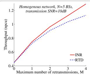
Figure 4 Throughput of the CoMP setup for different number of retransmissions M. Homogenous network, N=5, transmission SNR = 10 dB.
