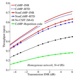
Figure 1 System throughput vs the transmission SNR 10  $\log_{10} P$ . Homogenous network  $\lambda=1$ , N=4 BSs, a maximum of M=1 retransmission rounds for the HARQ protocols.
