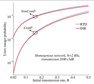
**Figure 2** User outage probability vs the initial transmission rate R. Homogenous network  $\lambda = 1$ , N = 2 BSs, SNR = 5 dB, a maximum of M = 1 retransmission rounds for the HARO protocols.
