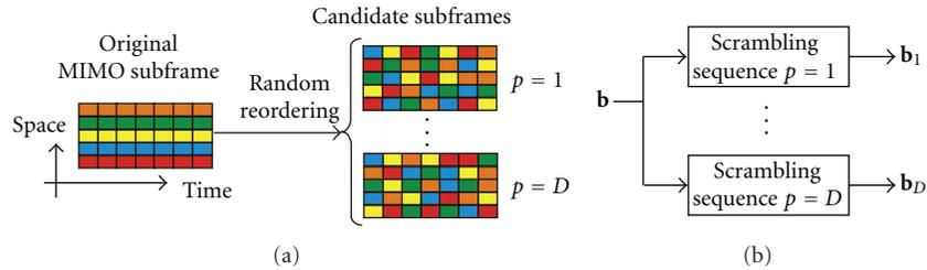
FIGURE 2: Mapping methods: (a) symbol reordering, (b) symbol scrambling.
