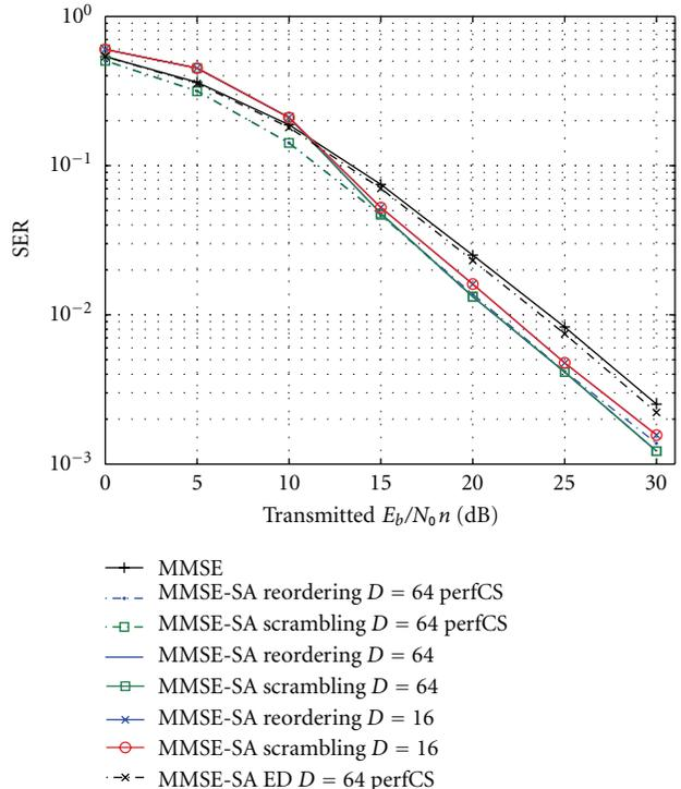
FIGURE 8: SER versus SNR for MMSE, MMSE-SA with reordering or scrambling, projection-based optimisation and MMSE-SA with Euclidean distance (ED) optimisation  $N = M = 5$ ,  $N_t = 7$ , QPSK.
