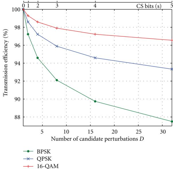
FIGURE 7: Transmission-reception efficiency for SA for increasing  $D$ ,  $N = M = 5$ ,  $N_t = 7$ , QPSK.
