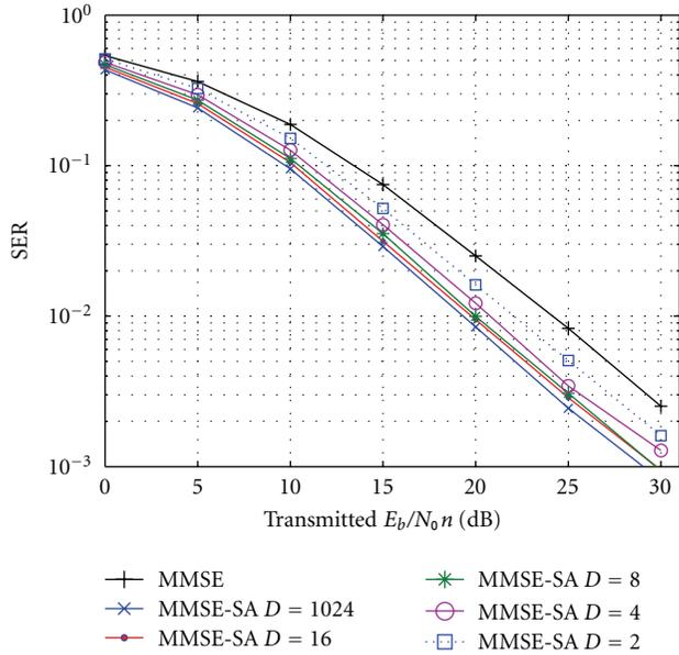
FIGURE 5: SER versus SNR for MMSE, MMSE-SA for increasing  $D$ ,  $N = M = 5$ ,  $N_t = 1$ , QPSK.
