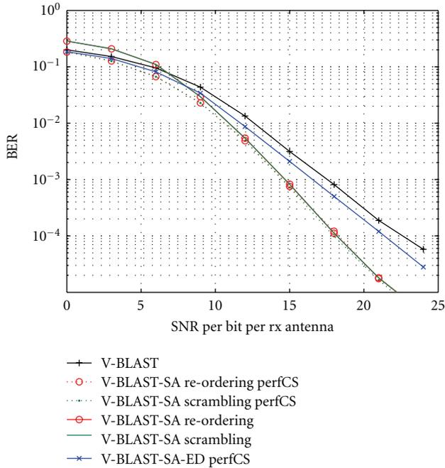
FIGURE 9: BER versus SNR for V-BLAST, V-BLAST-SA with reordering or scrambling, projection-based optimisation and V-BLAST-SA with Euclidean distance (ED) optimisation  $N = M = 5$ ,  $N_t = 7$ ,  $D = 16$ , QPSK.
