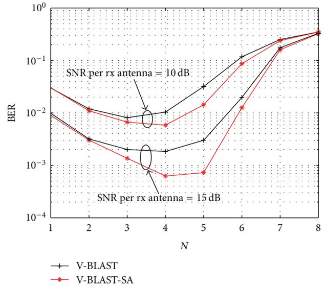
FIGURE 10: BER versus  $N$  for V-BLAST, V-BLAST-SA for SNR per rx antenna = 10 dB and 15 dB,  $N = M$ ,  $N_t = 7$ , QPSK.
