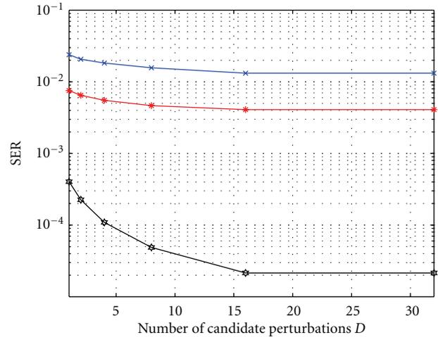
FIGURE 6: SER versus  $D$  for MMSE (SNR = 20 dB, 25 dB) and V-BLAST (SNR per rx antenna = 20 dB) using SA,  $N = M = 5$ ,  $N_t = 7$ , QPSK.
