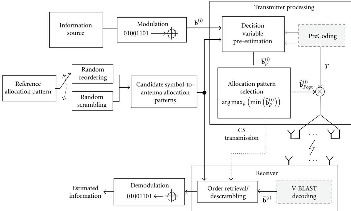
FIGURE 1: Block diagram of the proposed symbol allocation (SA) scheme.
