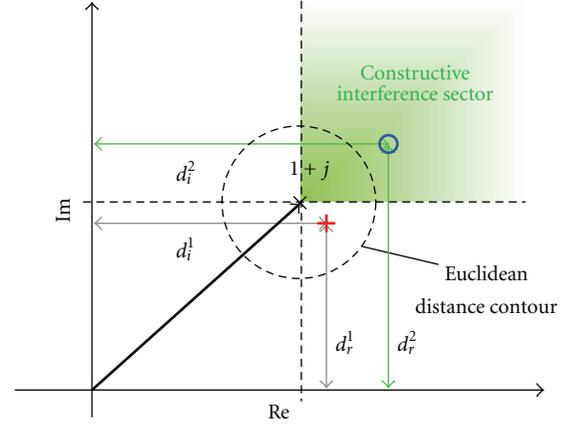
FIGURE 3: Euclidean distance versus projection criterion, QPSK  $x = 1 + j$  example.
