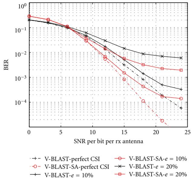
FIGURE 11: BER versus SNR for V-BLAST, V-BLAST-SA for CSI errors  $e = 0$ ,  $e = 10\%$ ,  $e = 20\%$ ,  $N = M = 5$ ,  $N_t = 7$ ,  $D = 16$ , QPSK.
