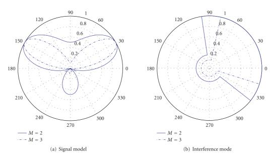
FIGURE 2: A simplified beamforming model with arrival angle  $\theta = 30^{\circ}$ .
