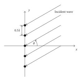
FIGURE 1: ULA antenna array.
