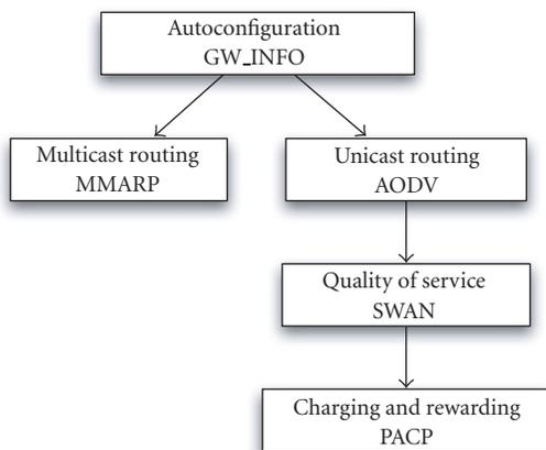
FIGURE 3: Functional architecture with protocols included.
